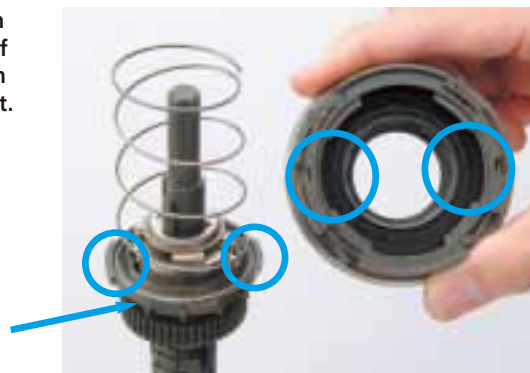
Set drive unit while turn it counterclockwise.
